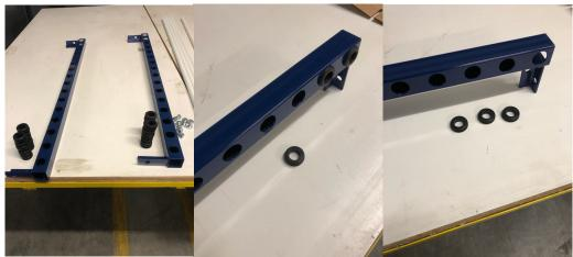
Start by adding the grommets into the holes on the sides of the frames. A small flat head screwdriver will help with the installation of the grommets.
