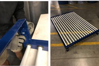
Take the other metal piece (no holes) and install it by sliding the end piece down over the other metal piece. Secure the two metal pieces together with the nut and bolt provided. There should be eight nuts and bolts pr section. Do this to both sides.
