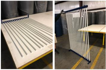
Lay the one metal frame piece that has holes in it, on the ground or table, with the metal end pieces sticking up. Insert the fiberglass rods into each hole. There should be 16 rods. Install the other side in the same manner. The metal frame piece should stay in place
